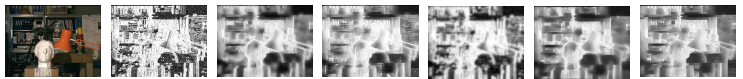
An inferred matching probability in 'Tsukuba' image when the candidate of disparity is 0. (From left to right) Original image, initial matching cost, Adaptive weight (AW) [2], Cost filter (CF) [3], Anisotropic diffusion (AD) [4], Geodesic diffusion (GD) [5], and (e) The proposed method. The low intensity indicates high probability of being matched, and vice versa.
