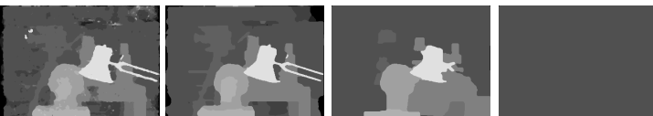
Disparity estimation results of the proposed method when the restarting probability is (from left to right) 3 \times 10^{-1} , 3 \times 10^{-2} , 3 \times 10^{-3} , and 3 \times 10^{-4} . As the restarting probability approaches to zero the results becomes constant, i.e. it has no meaningful solution.
